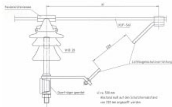
Picture 7. Mounting instruction of the arcing horn system.
